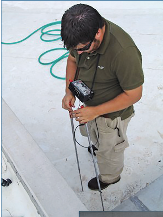
Figure 20 - Using potentiometer to discover source of leaks.
