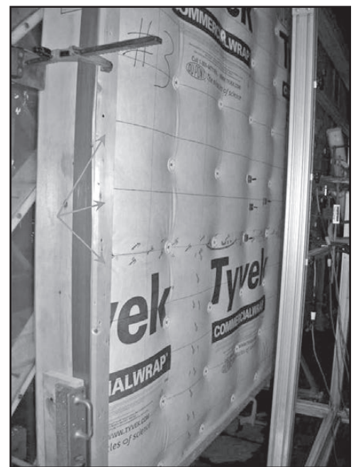
Figure 2 – High-pressure testing of wall assemblies with mechanically fastened air barrier systems. Source: DuPont testing at ATI.
