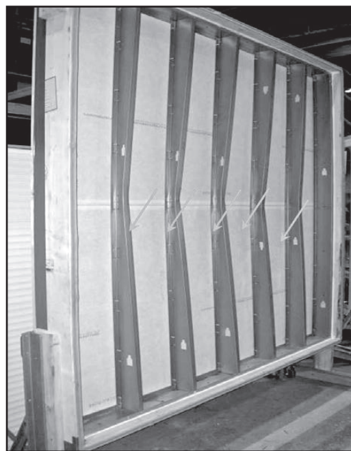
Figure 2 – High-pressure testing of wall assemblies with mechanically fastened air barrier systems. Source: DuPont testing at ATI.
