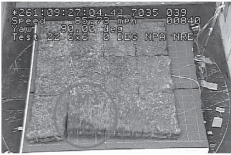
Failure initiated at M3
