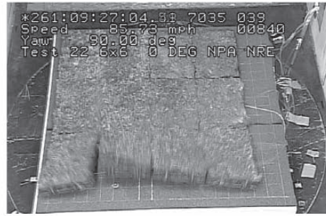
Figure 11 – Typical failure mode of 6 x 6 ft. NPE at 0-degree wind angle.
