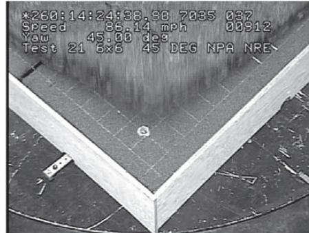
Figure 12 – Typical failure mode of 6 x 6 ft. NPE at 45-degree wind angle.
