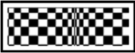
Figure 5. Representative reflected image of a checkerboard on distorted heat-treated glass.
