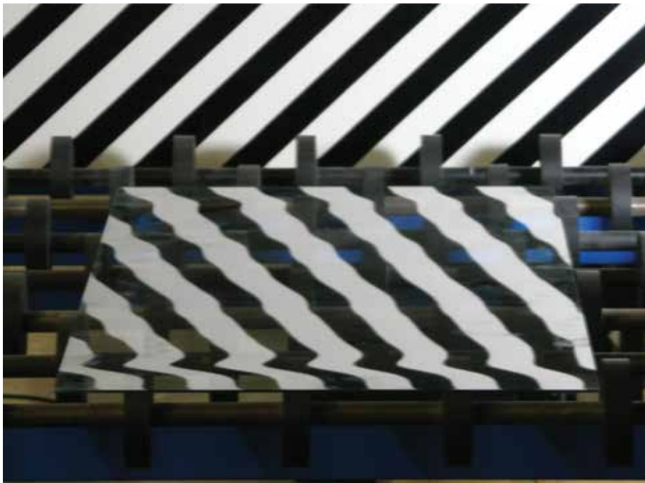
Figure 1. Zebra board visual evaluation of glass distortion on heat-treated glass.
