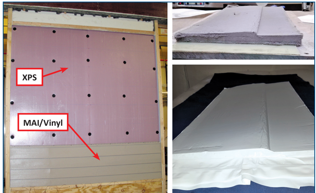
Figure 5 – Fabrication of MAI panels and construction of the GHB test specimen.
