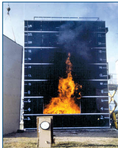
Figure 2 – View (front) of the two story, exterior wall apparatus during a fire test. Earlier versions of the NFPA 285 test were conducted outside. Courtesy of Jensen Hughes.
