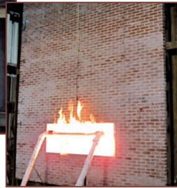
Figure 2. Two-story test with interior and exterior burners.
