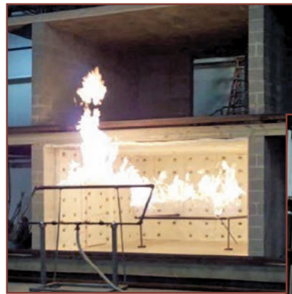
Figure 2. Two-story test with interior and exterior burners.
