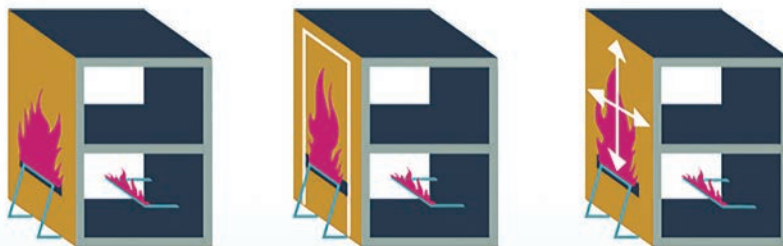
Figure 3. NFPA 285 4 fire test parameters and pass criteria.
