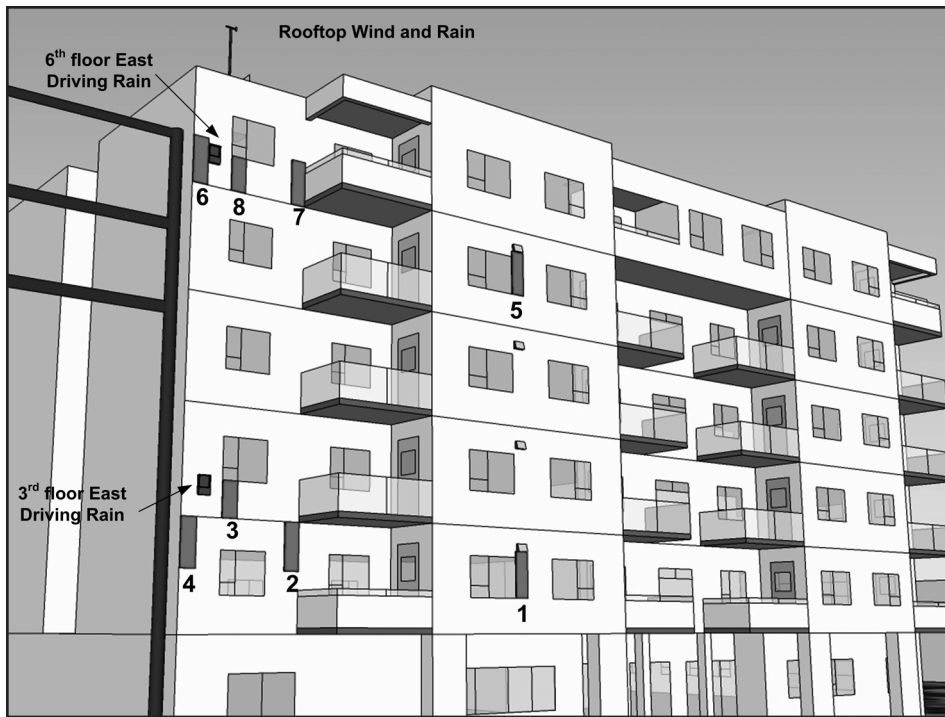
Figure 2 - Building 3 of the monitoring study, location of monitored walls and sensors.
