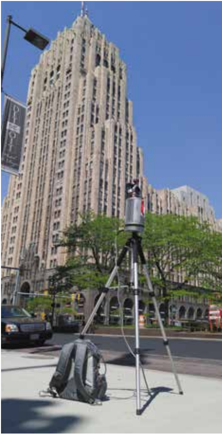
Figure 3. Laser Scanning utilized during assessment.
