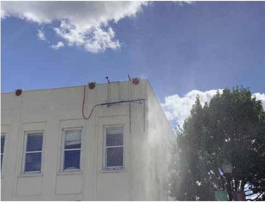
Figure 8. Representative view of Modified ASTM E1105 testing of mass masonry.
