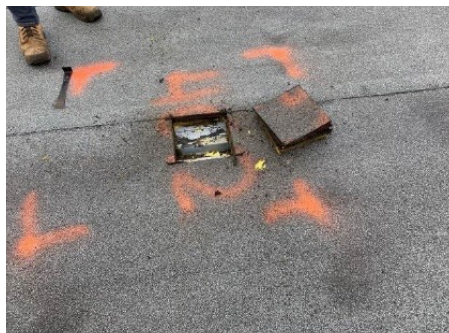
FIGURE 10. Cut test verification of roof assemblies – Pretium Eng. project
