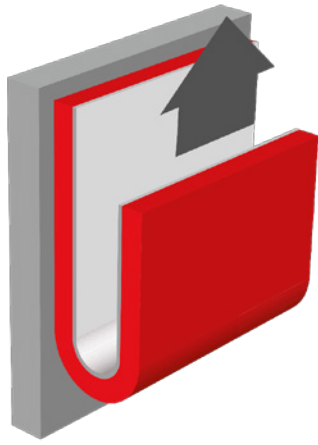
FIGURE 3. Typical 180-degree peel adhesion. (Courtesy of tesa tape Inc.)
