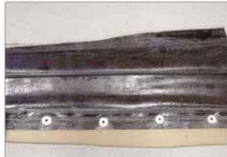
Figure 11. Membrane pullout from the fastener plate in mechanically attached roofing system.
