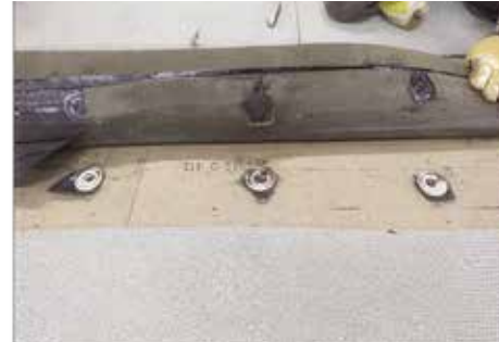
Figure 11. Membrane pullout from the fastener plate in mechanically attached roofing system.
