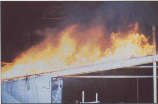
Photo 1: The ASTM E108 spread of flame test is carried out by Factory Mutual.
