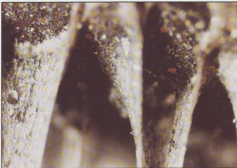
Photo 4: Light microscope examination of adhesive “legs” within lap splice. This is an example of qualitative testing, there being no measurements.
