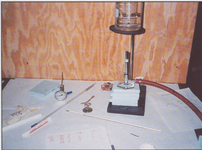
Photo 1: A softening point test underway. Often confused with "melt point," there is no relationship between these properties.
