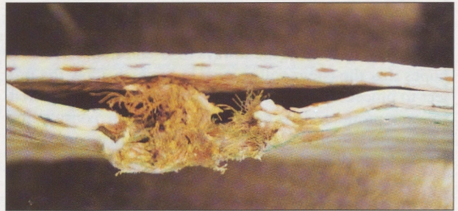
10. (Top) Another example of green food dye traveling through capillaries. 11. (Bottom) Edge of membrane at fastener hole. Note the frayed reinforcing fabric.
