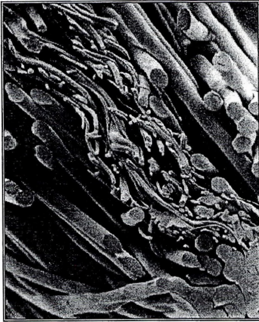
Figure 4—An example of three-layer, breathable membrane for use in roof and wall applications.
