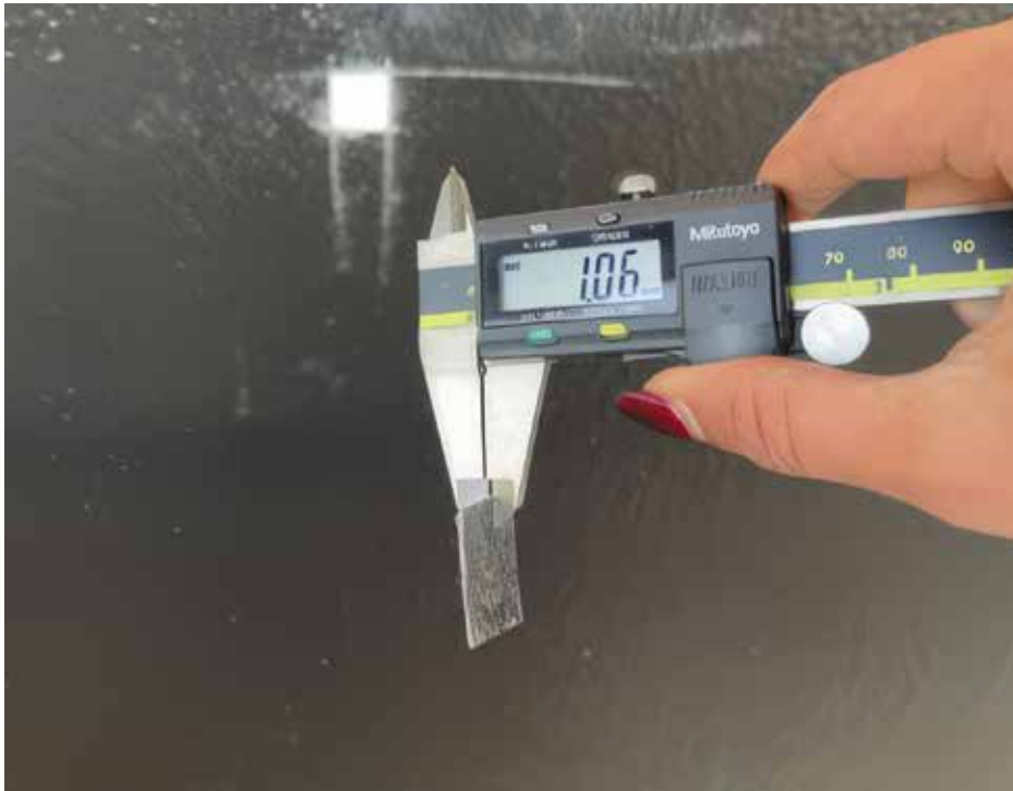
Figure 6. Passing result in the dry film thickness test.
