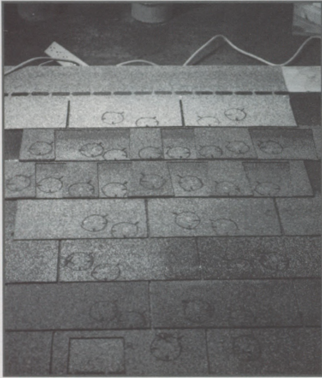
Overview of shingle test assembly
