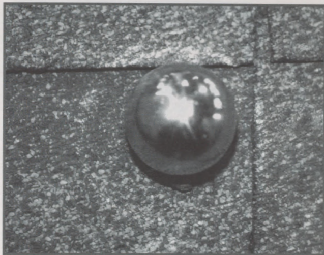
View of steel ball at impact location
