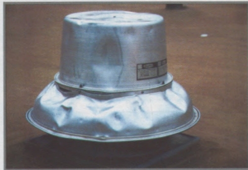
Figure 7A (left): Polyurethane-coated SPF roof system impacted by "oversize" hail in Big Springs, Texas. The average indentation diameter was almost 2.7 inches (210% bigger than the indentation created by FM-SH golfball-size (1.3 inches) hail impact). Figure 7B: HVAC unit showing the indentations created by "oversized" hail in Big Springs, Texas (May, 1996).
