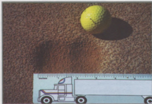
Figure 7A (left): Polyurethane-coated SPF roof system impacted by "oversize" hail in Big Springs, Texas. The average indentation diameter was almost 2.7 inches (210% bigger than the indentation created by FM-SH golfball-size (1.3 inches) hail impact). Figure 7B: HVAC unit showing the indentations created by "oversized" hail in Big Springs, Texas (May, 1996).
