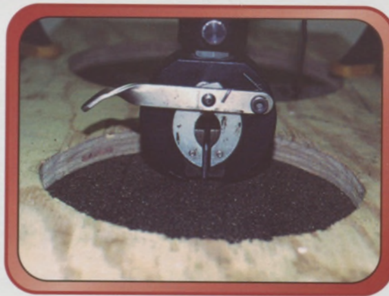
Figure 10 (left): View of FMRC Rupture Test (7" diameter).
