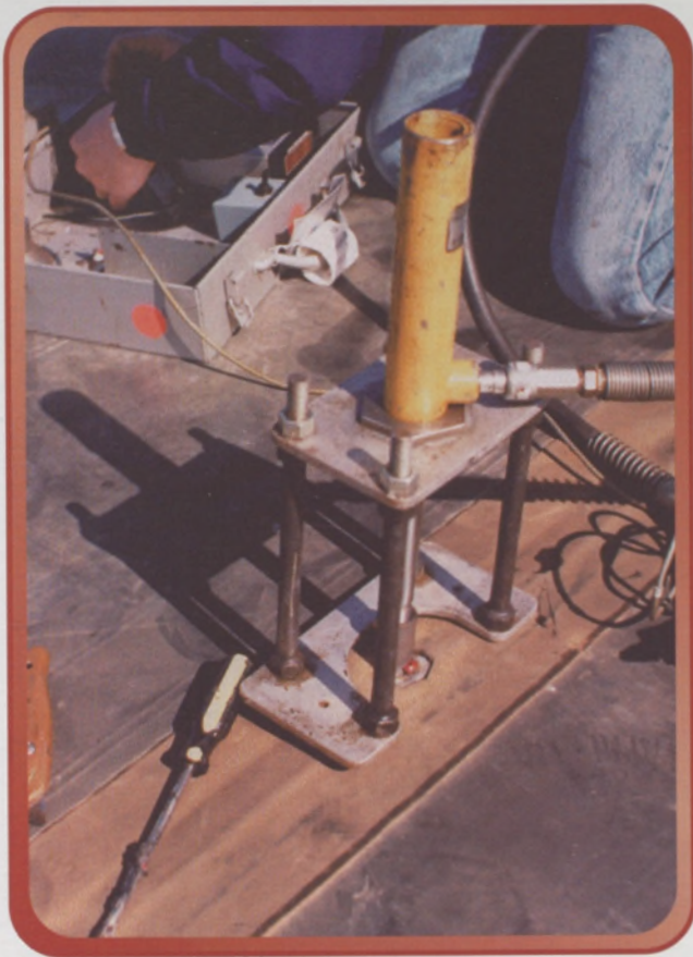
Figure 3: View of Field Withdrawal Resistance Testing
