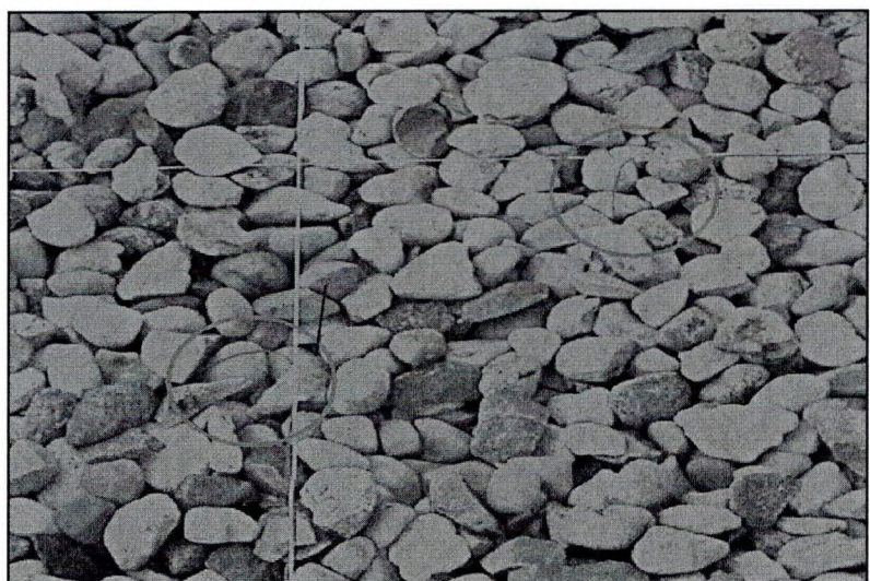
Figure 4 – Thermocouple measuring junctions placed against pieces of stone at the top of the stone-ballasted test sections.
