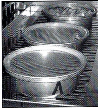
Figure 6 – ASTM E 96 cup test samples.
