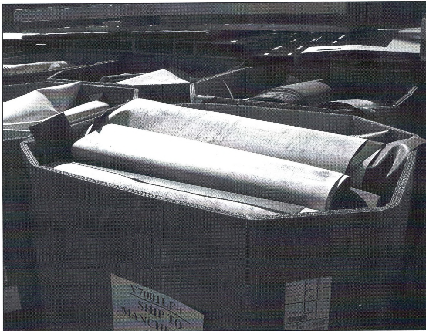
Figure 6 - PVC membrane packaged for shipping to recycling plant.
