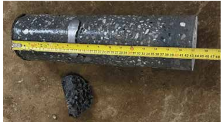
Figure 10. Extracted core from foundation wall showing reinforcement bar shadowing.
