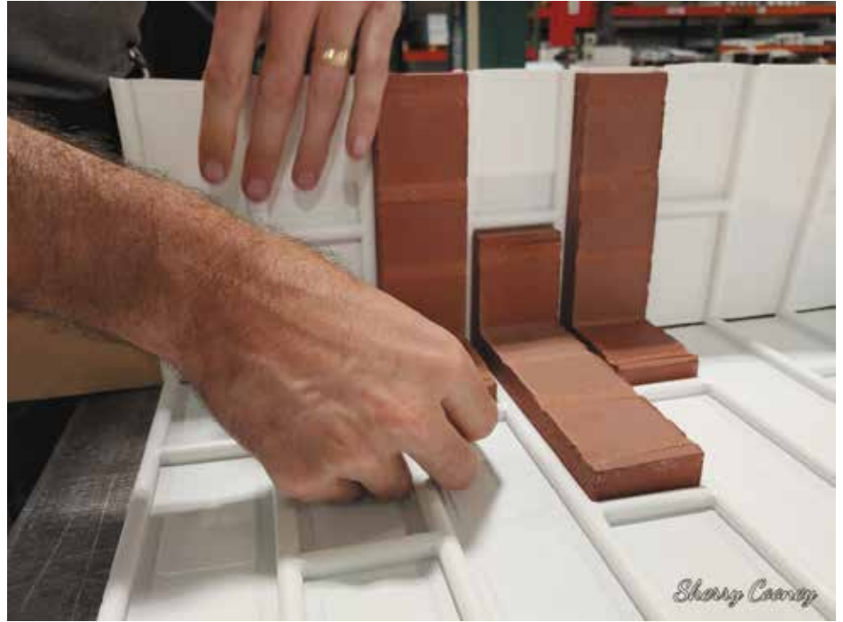
Figure 2b. Returns are cast into precast concrete thin brick panels by utilizing specialty form liners and bricks, as shown in this photo.
