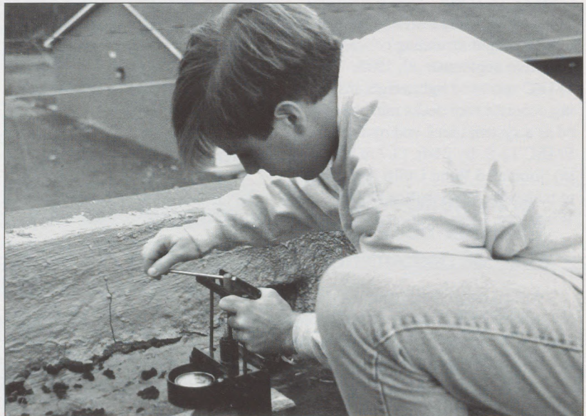
Mike Merrigan, of Olympic Fasteners, performs a pull test on the deck of the Pembroke municipal building being studied.
