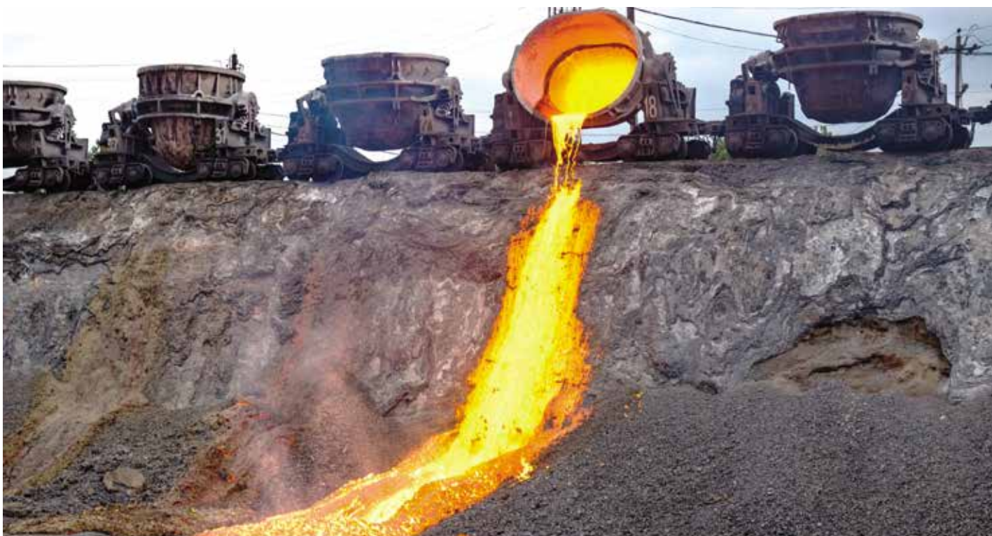
Figure 5. Blast-furnace slag is what is left over when, in the smelting process, pure steel is separated from impurities. This is in contrast with other aggregates that are mined (that is, blasted from a quarry) or those dredged from a river bottom (that is, stone ballast). Courtesy of DepositPhotos.com.
