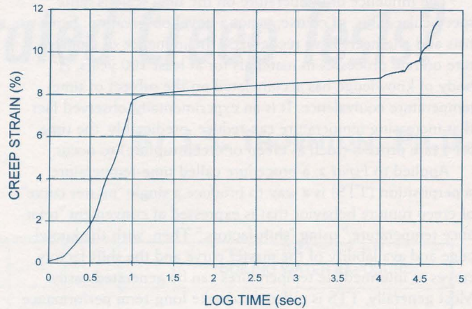
Figure 7. The creep data of Figure 4 plotted vs. log time.
