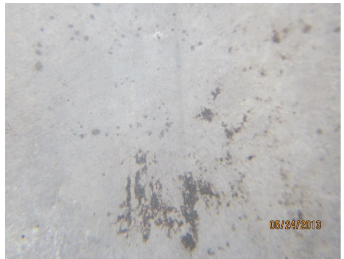
Figure 13. Photograph of a cleaned hail-caused dent under 10x magnification—note the absence of evident corrosion.
