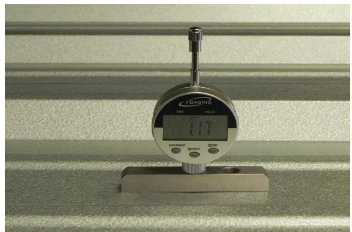
Figure 3. A field dent depth measurement.
