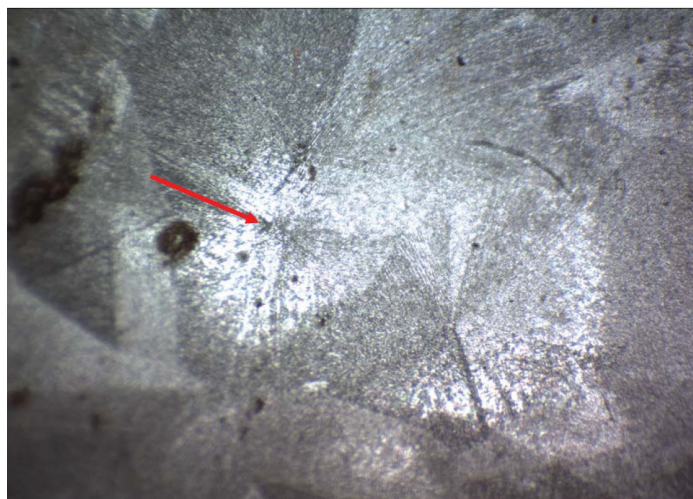
Figure 5. A view of a 1.75-inch steel ball impact point center under 80x magnification. The red point indicates a coating scuff.
