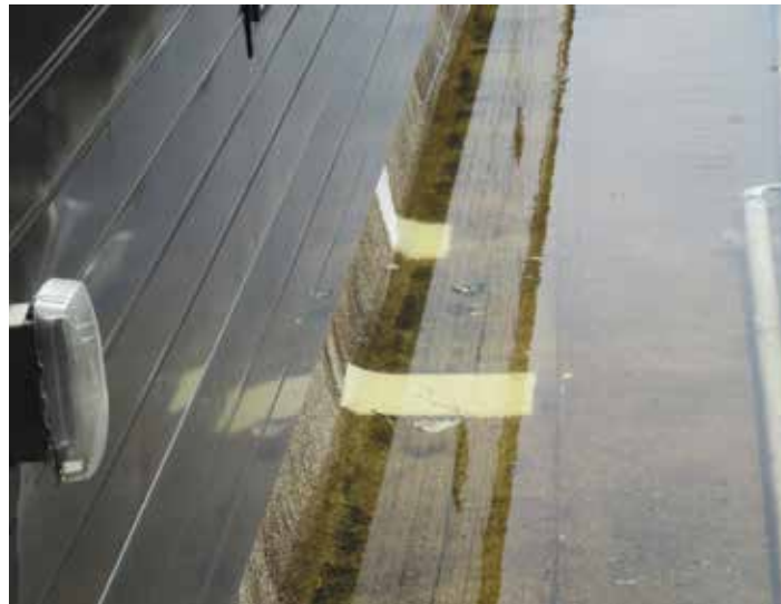
Figure 12. Minor deficiencies patched with polymethyl methacrylate membrane, after which the southeast vegetative area was separately tested, resulting in a third replication of the leak (3/19/2020).
