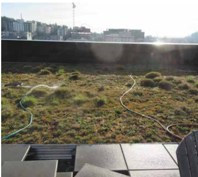
Figure 9. The southeast-corner vegetative roof was saturated with water, replicating the leak for the second time (3/17/2020).
