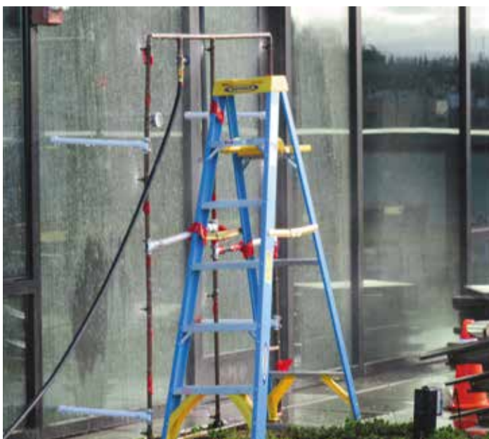
Figure 13. A spray rack was used to determine if the interface between the glazing assembly of the penthouse and the base flashing membrane of the roofing system contributed to the roof leak (3/23/2020).
