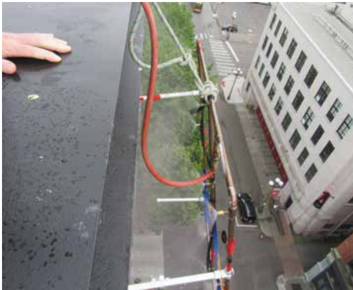
Figure 15. Spray rack was used to water test the exterior face of the south building parapet (5/20/2020).
