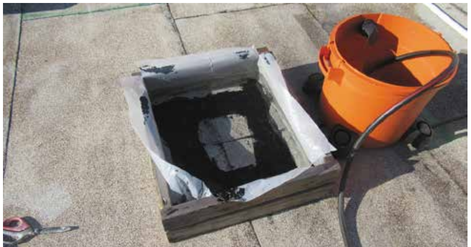
Figure 19. Flood test performed at a T-lap location suspected of being compromised (7/29/2020).
