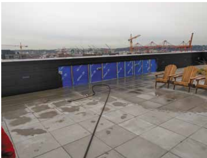
Figure 3. Eighth-floor parapet water tested with a calibrated spray wand shortly after the building was occupied with metal panel cladding removed to identify potential leak path(s) (2/11/2016).
