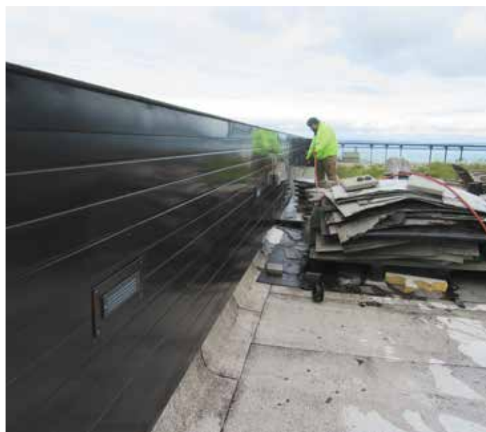
Figure 14. The south building parapet was tested using a calibrated spray wand at the base of the parapet, the metal cladding of its interior face, and the coping, in sequence from bottom to top (5/19/2020).
