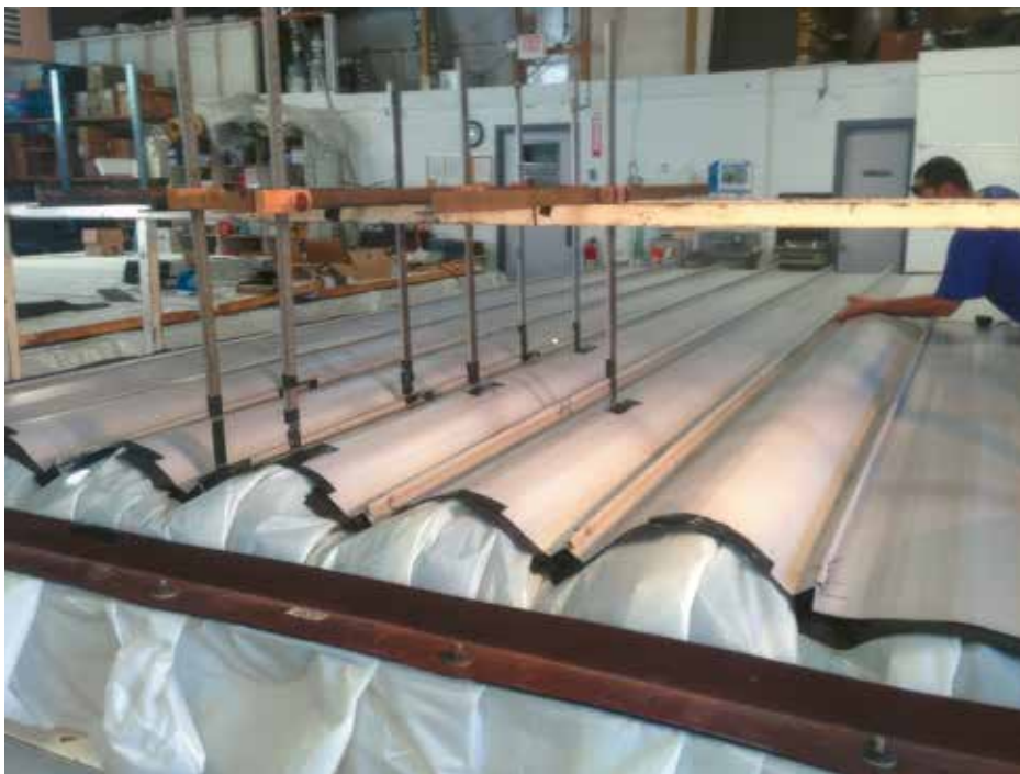
Figure 5. Performing ASTM E1592, Standard Test Method for Structural Performance of Sheet Metal Roof and Siding Systems by Uniform Static Air Pressure Difference, on panels mounted on notched zeeps.
