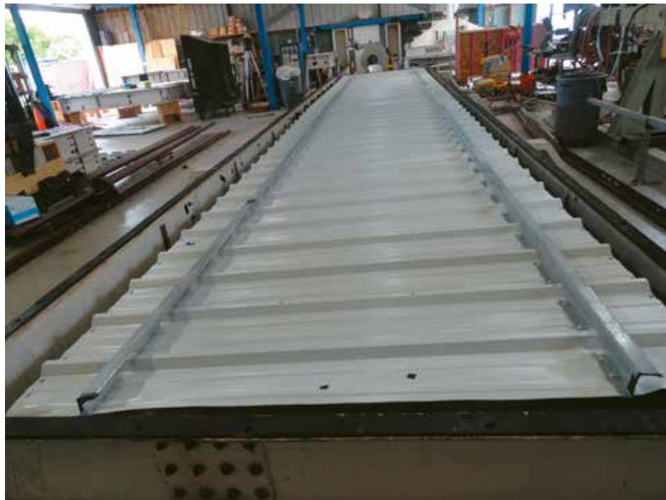
Figure 6. Gravity load base test of continuous purlins in 50-ft (15-m) long test chamber before applying loads according to AISI S908.
