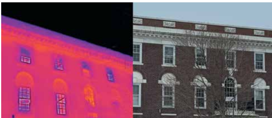
Figure 7. Air leakage at a mass masonry wall to roof transition.
