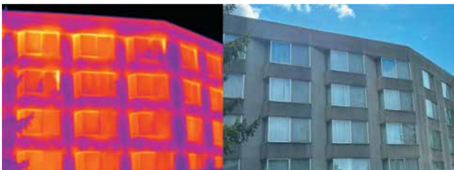
Figure 1. Thermal anomalies across the precast concrete building's facade.
