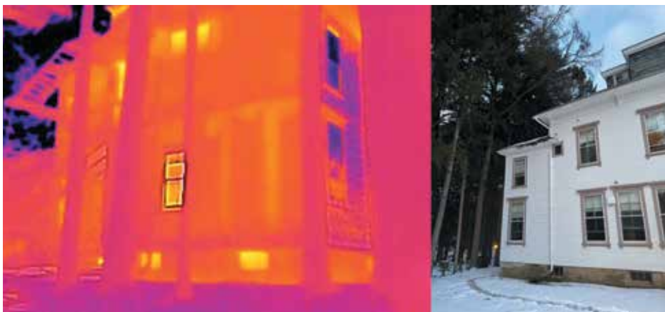
Figure 4. Missing bays of insulation at a wood-framed building.
