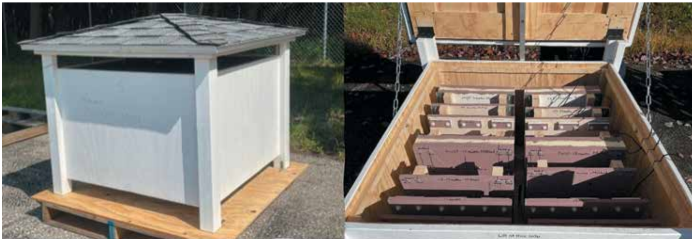
Figure 1. Small test hut used to house various panel configurations containing magnesium oxide boards and expose them to local ambient conditions without direct exposure to rain, such as might be experienced in a vented air gap behind typical claddings. The bottom and top of the enclosure are open to allow airflow through the enclosure (left image), with a hinged roof assembly allowing access to the samples evenly spaced within the enclosure (right image).
