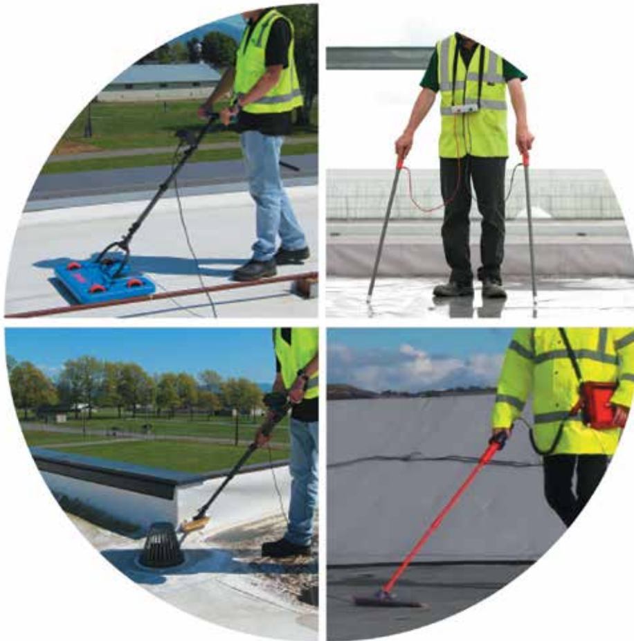
Figure 1. The four electronic leak detection methods.
