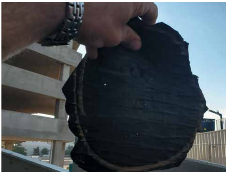
Figure 17. Example of clusters of breaches.
