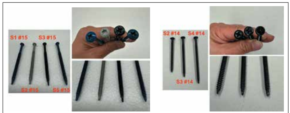
Figure 2. Fasteners evaluated for both static and dynamic.
