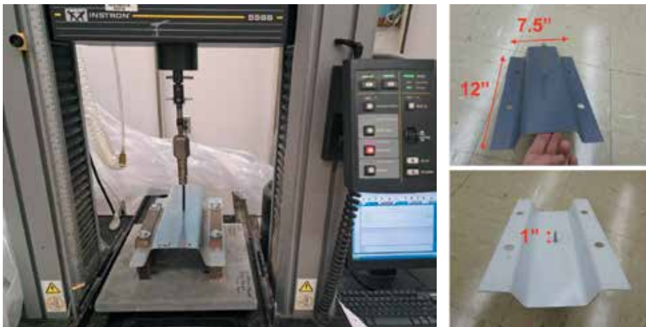
Figure 4. Setup for the static evaluation of the steel deck using the Instron.
