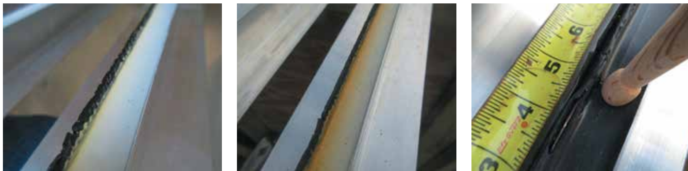
Figure 7. Photo examples of sealant at: (a) Week 6, slight yellow discoloration at Condition W-F, (b) Week 28, bright orange discoloration at Condition W-F, and (c) Week 28 with localized adhesive failure along edge in contact with bitumen-based waterproofing (Condition W-F).
