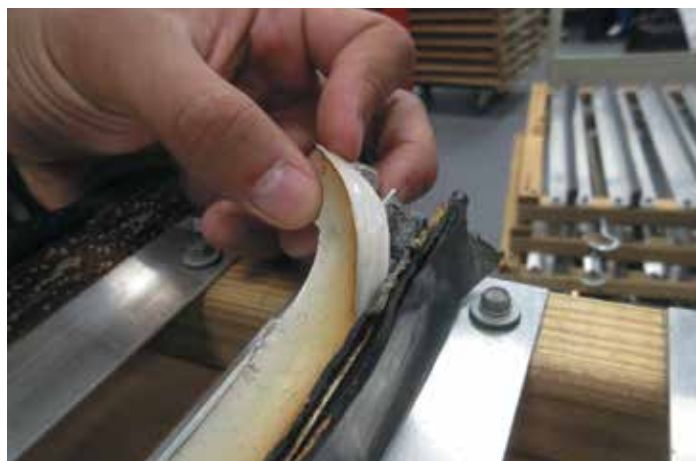
Figure 10. Top and side of sealant sample during extraction from the aluminum angles.
