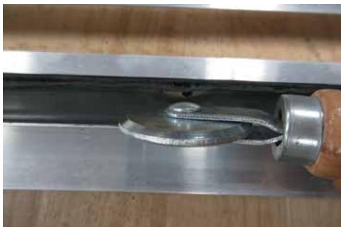
Figure 9. ASTM C1521 continuous nondestructive test at location of unadhered sealant.
