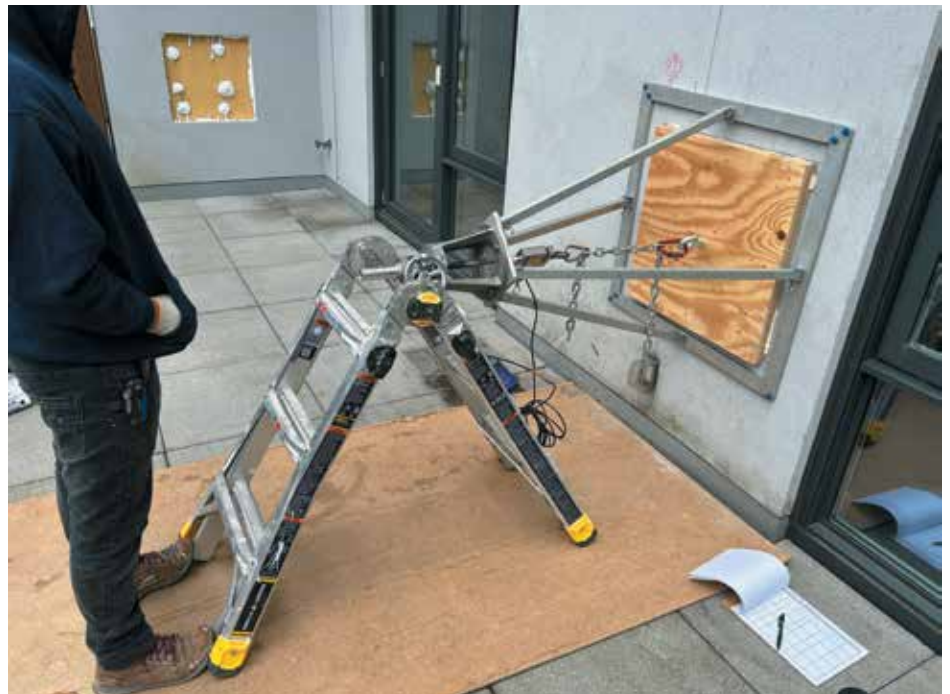
Figure 4. Exterior insulation and finish system adhesion testing.
