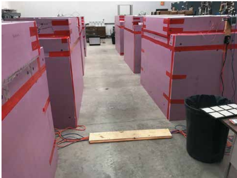
Figure 2. Photo of instrumented roofs over concrete decks at SRI's Middleton, WI, laboratory. Slabs were heated from below to 90°F (32°C) to provide a positive vapor gradient across the roof system.
