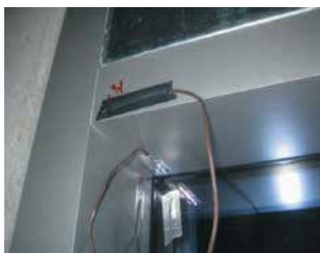
Figure 4. Thermocouple datalogger leads at the surfaces of an insulated glass unit and mullions.
