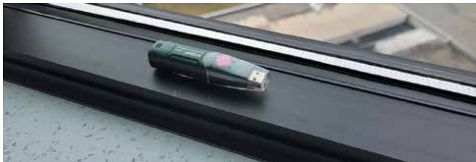
Figure 3. Temperature and humidity datalogger on a windowsill.
