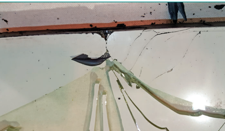
Figure 3 – View of the back side of the spandrel IGU in Figure 2, after it was removed from the curtainwall. The crack split toward the center-of-glass area, as seen in Figure 2 and also to the edge of the inboard pane, indicating the origin of the crack was inward from the edge.
