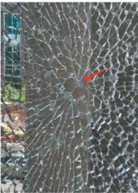
Figure 1. View of shattered glass indicating butterfly pattern.
