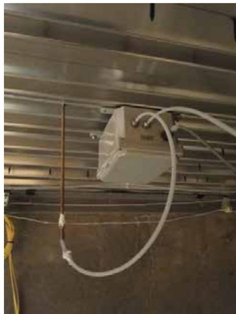
Figure 2. Details of the pressure sensor developed by National Research Council of Canada to evaluate wind load on the roof. Note: DAQ = data acquisition system.
