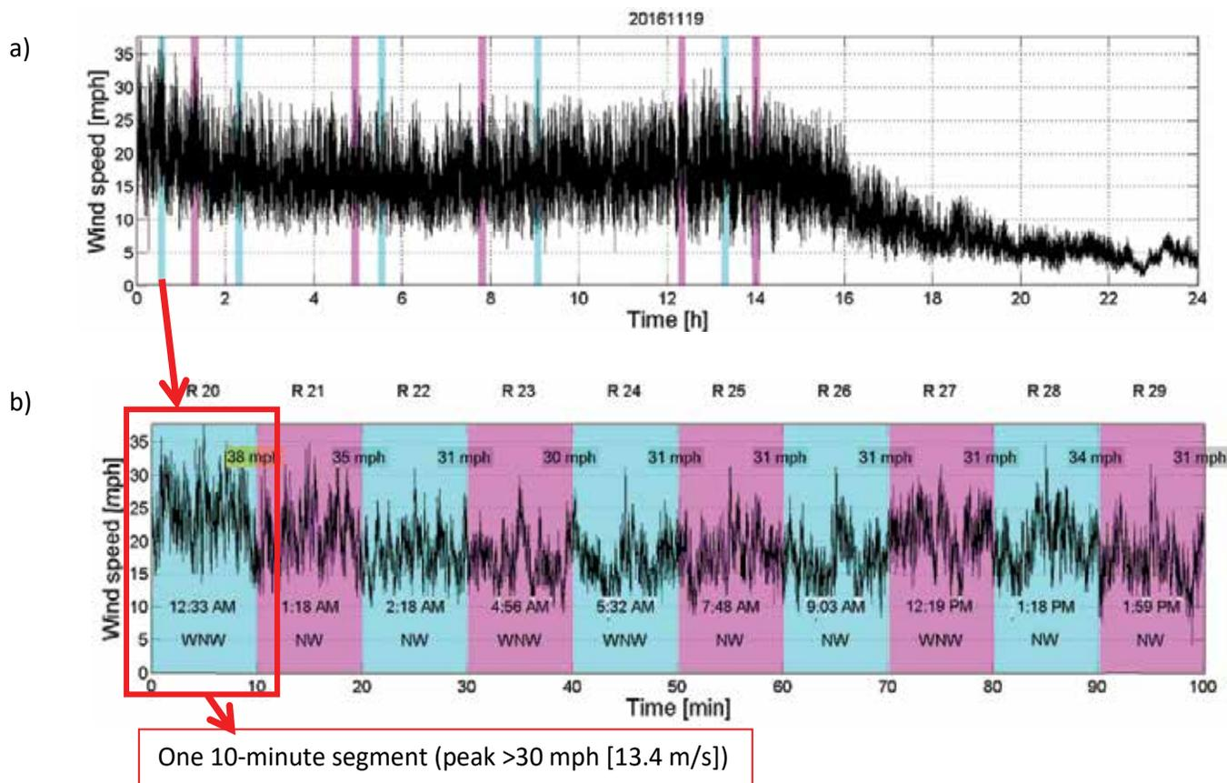
**Figure 3.** Data from field monitoring: (a) typical wind speed time history; (b) example of data segmentation into 10-minute records (November 19, 2016). Note: 1 mph = 0.447 m/s.
