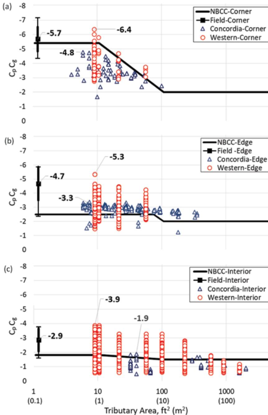
**Figure 5.** NBCC provisions versus wind tunnel and field data (a) corner, (b) edge, and (c) interior. Note: NBCC = National Building Code Canada.<sup>1</sup>
