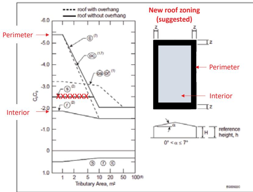
**Figure 6. NBCC provisions modified to illustrate the suggested new provisions and roof zones. Note: NBCC = National Building Code Canada.<sup>1</sup>**
