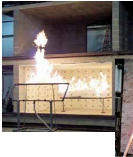
Figure 2. Two-story test with interior and exterior burners.
