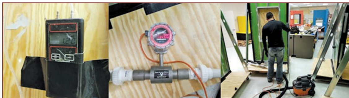
Figure 11. Air-leakage testing equipment (manometer, airflow meter, commercial vacuum).
