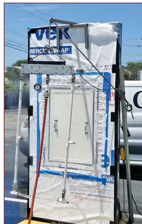
Figure 12. ASTM E1105 water testing of mock-up 2, round 1 testing.
