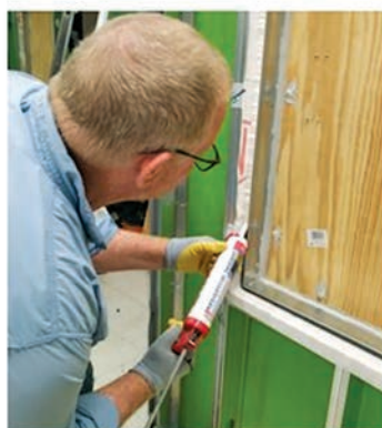
Figure 5. Mock-up 3, round 1 testing, mechanically fastened WRB system. Note: WRB = water-resistive barrier.
