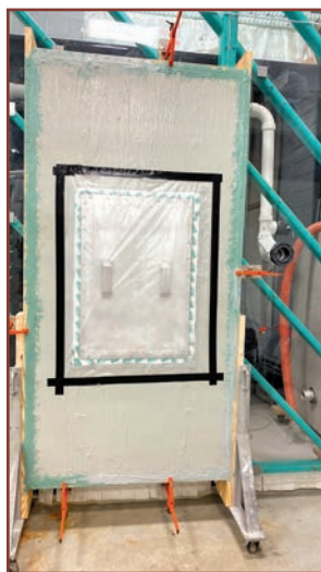
Figure 10. Mock-up 3, round 2 testing during blank isolation air-leakage testing.
