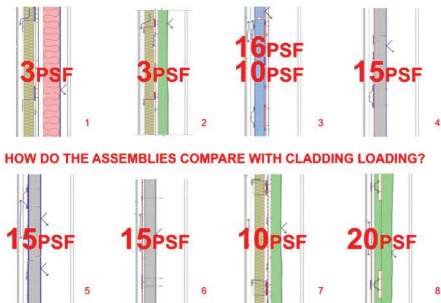
Figure 18. Comparison of cladding support loadings ranging from 3 to 20 psf.
