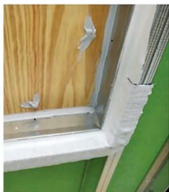
Figure 7. Mock-up 5, round 1 testing, mechanically fastened WRB system. Note: WRB = water-resistive barrier.
