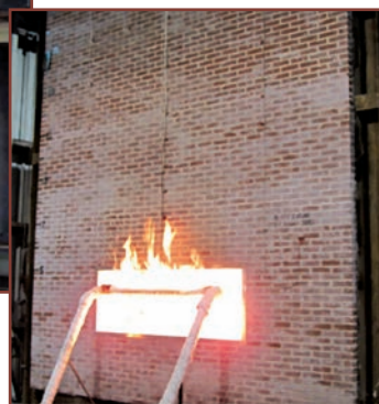
Figure 2. Two-story test with interior and exterior burners.
