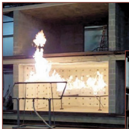
Figure 2. Two-story test with interior and exterior burners.
