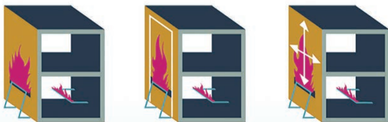
Figure 3. NFPA 285 4 fire test parameters and pass criteria.
