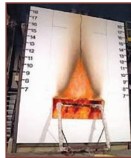
Figure 1. Stock image of NFPA 285 vertical and lateral fire propagation testing.
