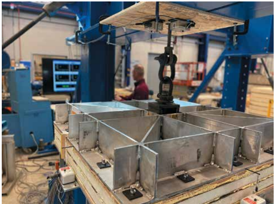
Figure 16. Application of axial load to a test specimen.
