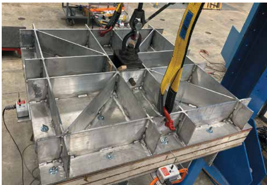
Figure 10. A stiffened aluminum test frame and secured insulation board test specimen.
