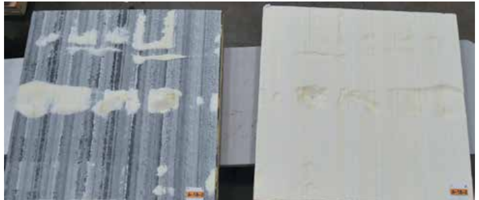
Figure 22. In specimen A-18-2, the primary failure was separation of the top facer of the bottom board from the foam core, with some cohesive bond separation within the foam core.
