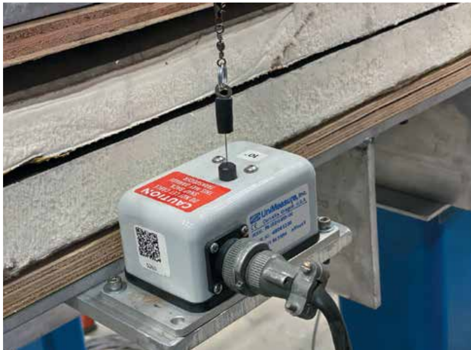
Figure 13. Displacement transducer positioned at the edge of a test specimen to measure separation and elongation of insulation during testing.
