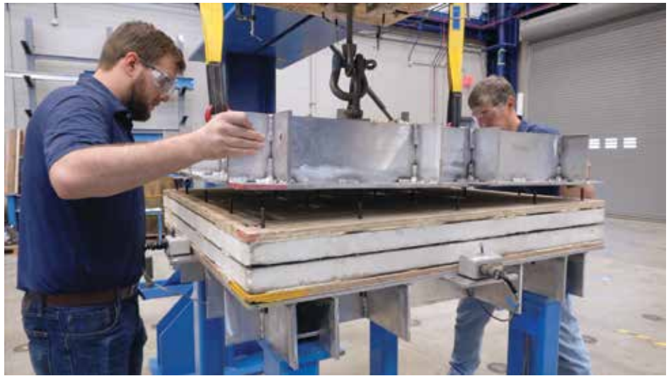
Figure 14. Positioning the upper aluminum load frame onto a test specimen.
