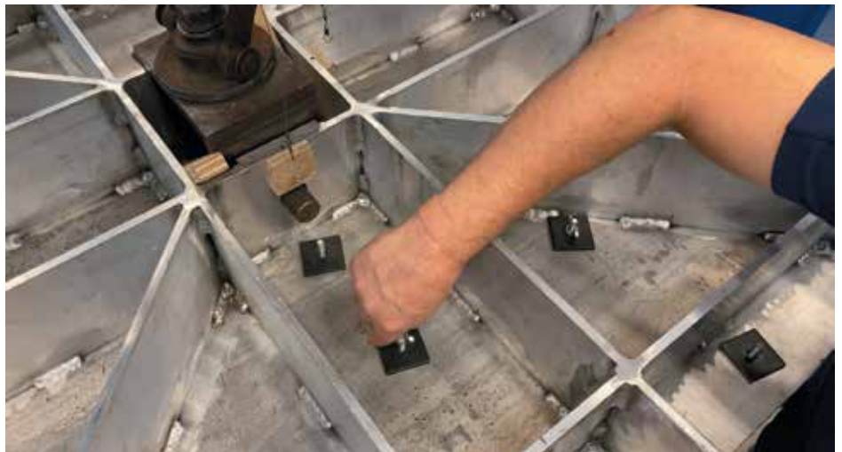
Figure 15. Securing the upper load frame to a test specimen with a plate and wing nuts onto threaded rods.
