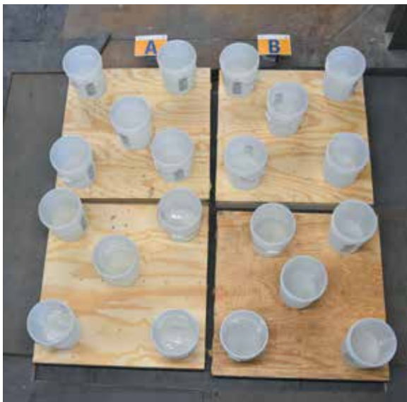
Figure 4. Typical weights used as ballast until the foam adhesive set up, typically for 10 to 15 minutes per specimen.
