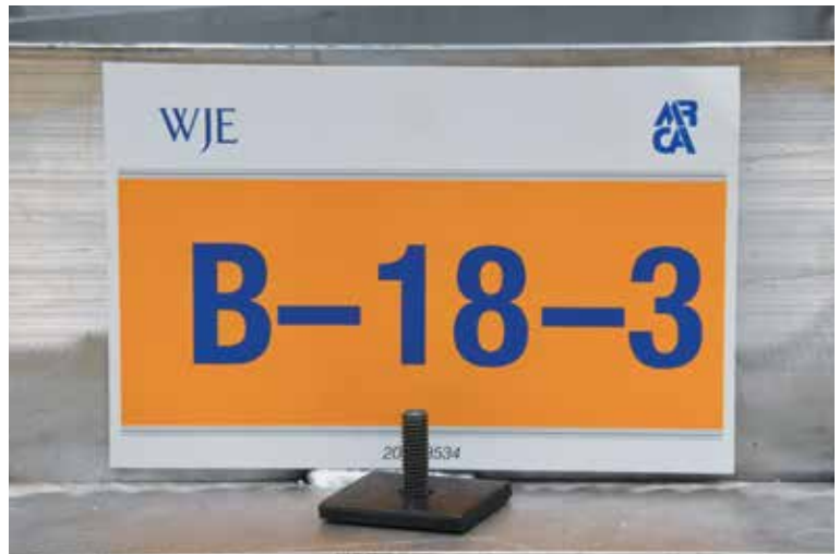
Figure 8. Example of the alphanumeric system and label used to identify the insulation specimens. B-18-3 indicates a cellulosic felt facer (B) with 18 in. ribbon spacing, and specimen number 3.
