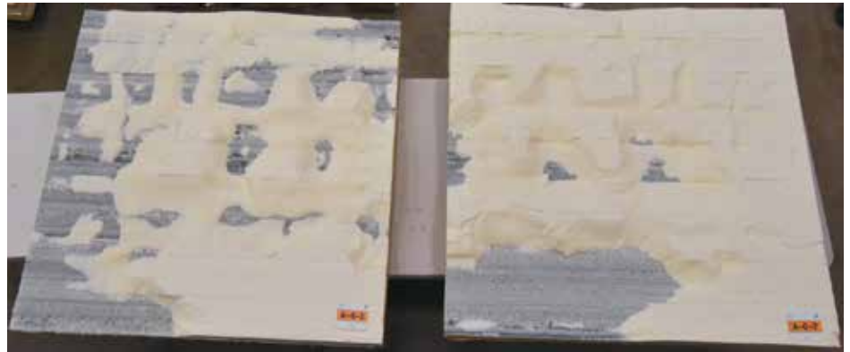
Figure 21. Specimen A-6-2 shown in separated fashion, similar to an opened book. The plane of failure was primarily within the foam core of the top facer of the insulation board (left), with some delamination at the bottom glass fiber facer of the board (right).
