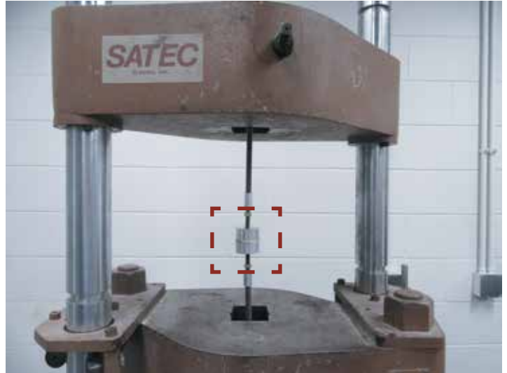
Figure 18. A 2-in.-diameter aluminum puck specimen with 1/8-in.-thick low-rise foam adhesive being tested in the hydraulic test machine.
