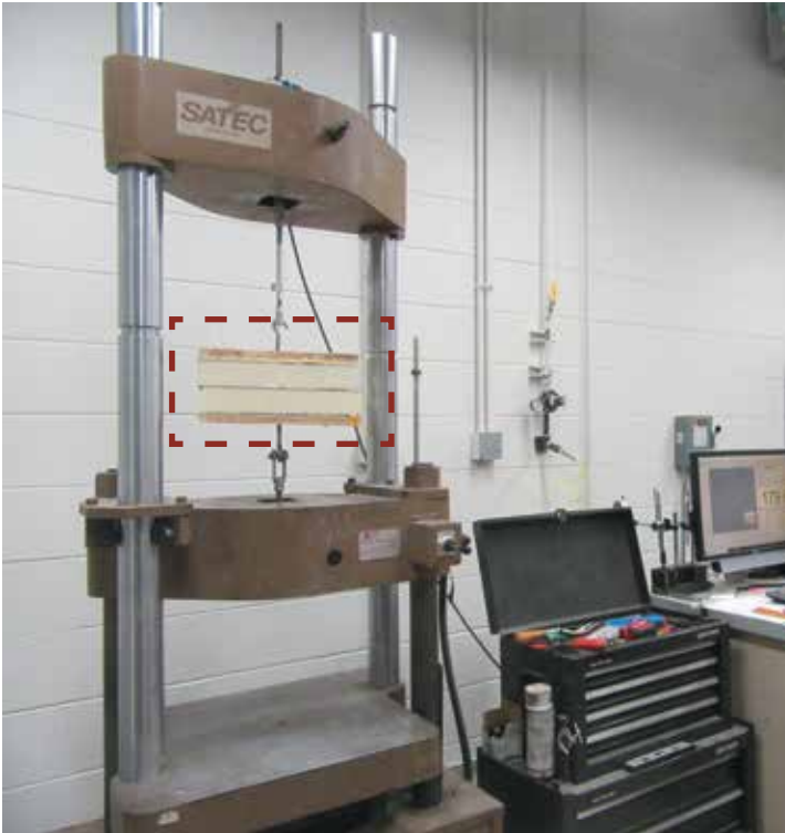
Figure 17. Testing of a 1 ft² insulation board specimen with a single ribbon of adhesive in the hydraulic test machine.
