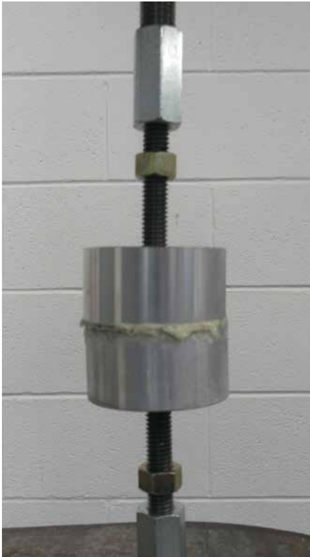
Figure 7. Two pucks with a 1/8-in.-gap space filled with foam adhesive.
