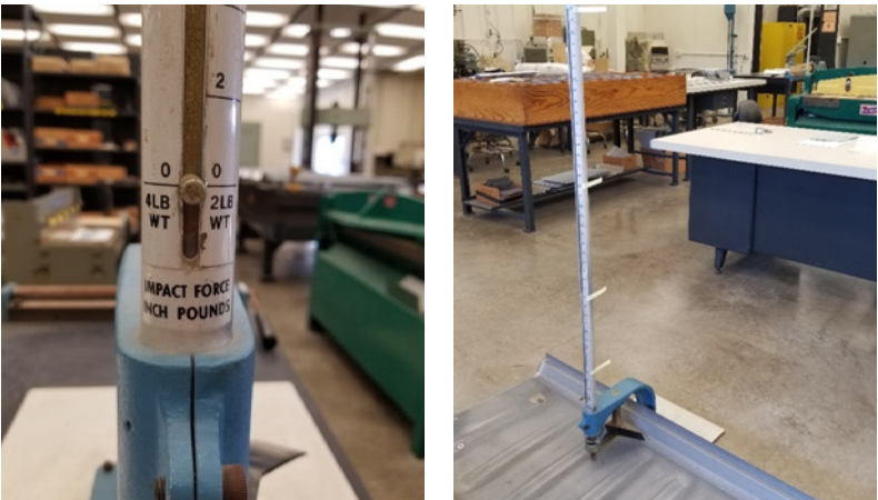
FIGURE 13. Impact test apparatus used to produce simulated hail divots in a Butler MR-24 panel.
