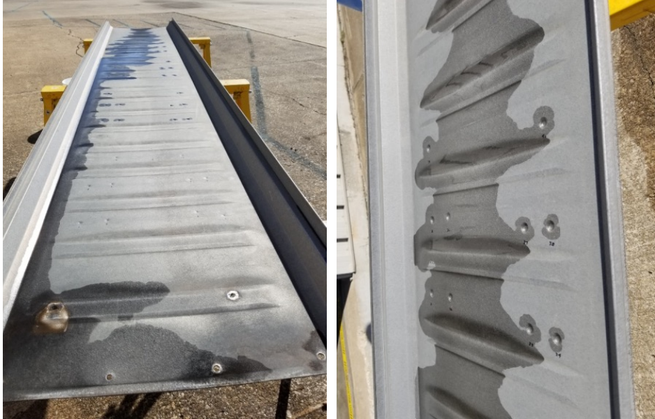
FIGURE 16. Non-uniform water distribution on panel as it dries (L) and subsequent effect on volume of water flowing into divots on the opposing sides of the panel (R).
