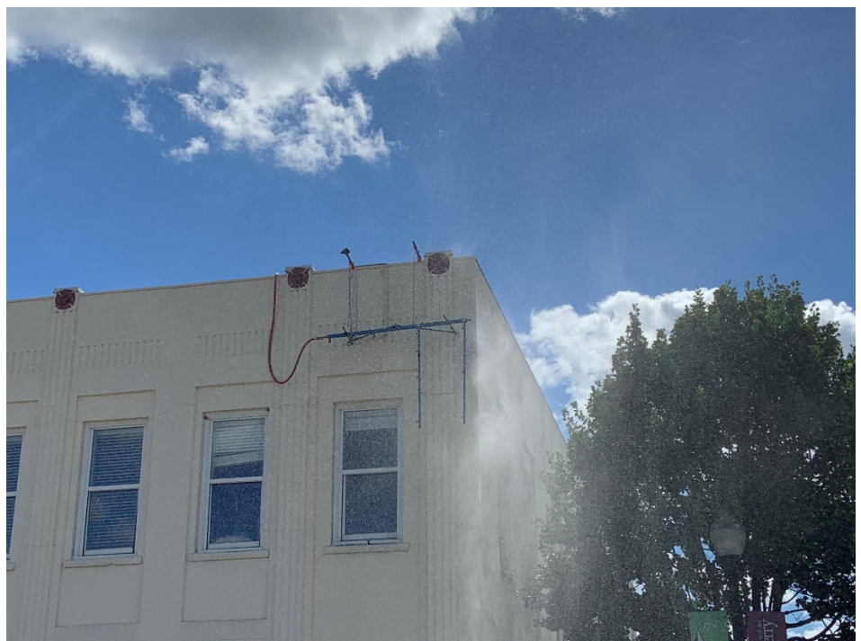
FIGURE 8. Representative view of Modified ASTM E1105 testing of mass masonry.
