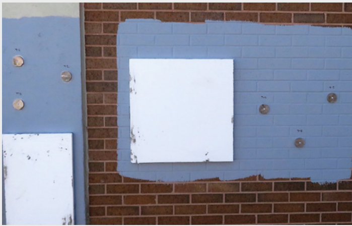
FIGURE 11. Mock-ups installed to evaluate adhesion of the AWB to substrates and the EIFS insulation to the AWB.
