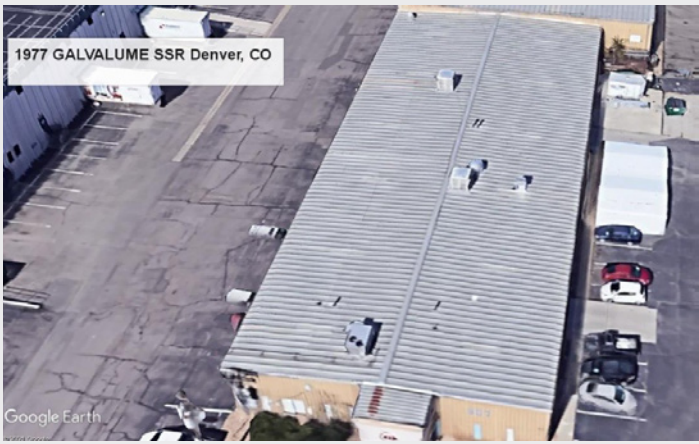
FIGURE 2. 55%Al-Zn alloy-coated steel SSR system erected in Denver, Colorado in 1977.
