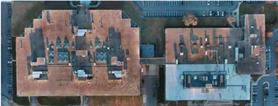
Figure 9. Fully stitched digital image of the roof.
