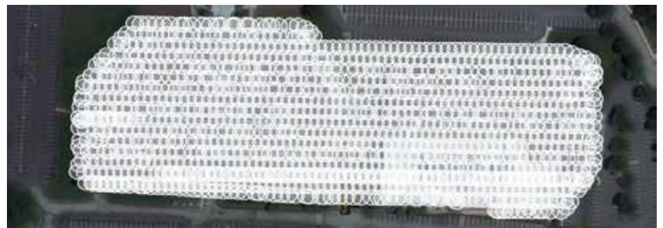
Figure 6. Image showing every photo taken during the mapping of a roof. Each white circle is one photo.
