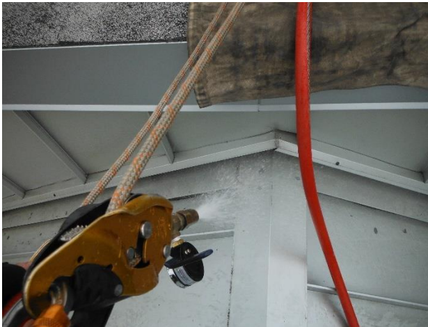
Figure 24. Water spray testing sidewall transition with missing counterflashing near ridge. Water intrusion observed after 5 minutes.
