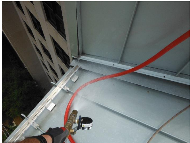
Figure 45. Water spray testing along sidewall transition at east side of gabled metal panel roof. No water intrusion observed.
