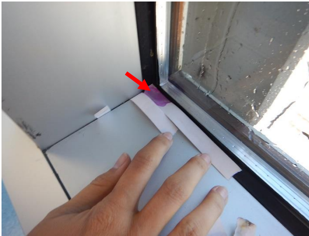
Figure 28. Water intrusion observed at gasket intersection at horizontal mullion below the test area.
