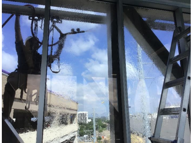
Figure 57. Water spray testing the vertical intermediate of a vision lite on the west facade of the skybridge near the Purple Garage. No water intrusion observed.
