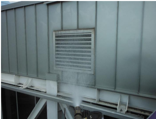
Figure 48. Water spray testing perpendicular to the west facade louver near the Purple Garage. Water intrusion observed after 2 minutes.
