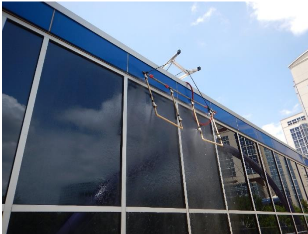
Figure 74. Spray rack testing of windows on north facade.
