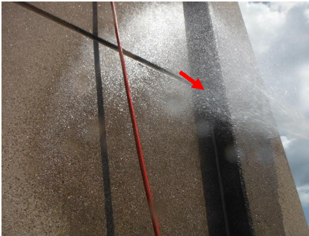
Figure 54. Water spray testing vertical sealant joint with adhesive failure above roof-to-wall transition at the elevator tower. Water intrusion observed after 4 minutes.
