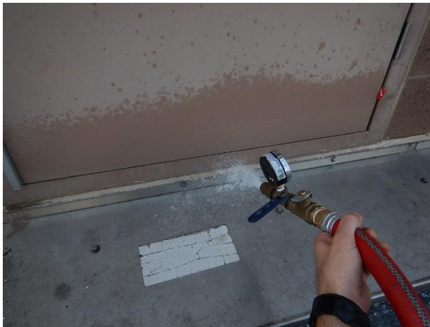
Figure 70. Water testing metal access door above roof-to-wall transition.
