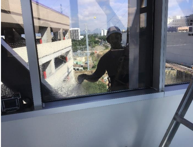
Figure 56. Water spray testing the horizontal intermediate of a vision lite on the west facade of the skybridge near the Purple Garage. No water intrusion observed.
