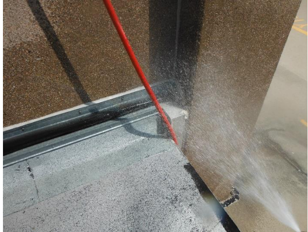
Figure 53. Water spray testing south end of roof-to-wall transition at the elevator tower for the Purple Garage. No water intrusion observed.
