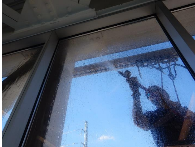
Figure 27. Water spray testing along window head.
