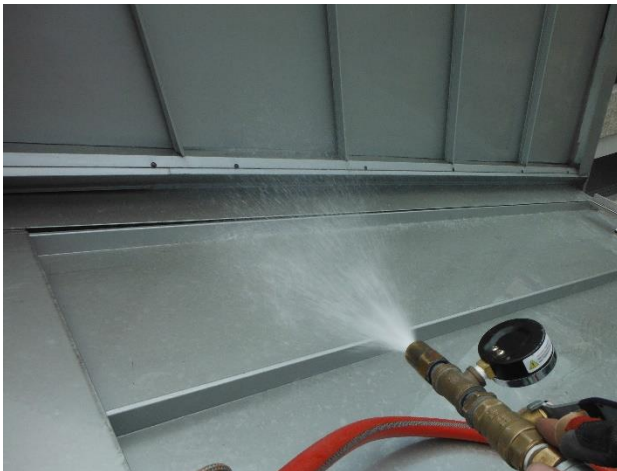
Figure 44. Water spray testing along sidewall transition at west side of gabled metal panel roof. No water intrusion observed.
