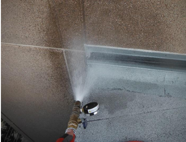
Figure 52. Water spray testing north end of roof-to-wall transition at the elevator tower for the Purple Garage. No water intrusion observed.
