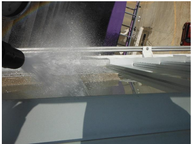
Figure 47. Water spray testing down onto the west facade louver near the Purple Garage. No water intrusion observed.
