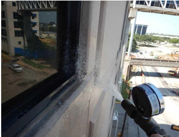
Figure 72. Water testing perimeter of 2nd floor window sill within Green Garage above roof-to-wall transition.
