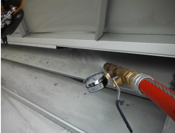
Figure 22. Water spray testing sidewall transition with missing counterflashing along south half of gabled roof. Water intrusion observed after 2 minutes.
