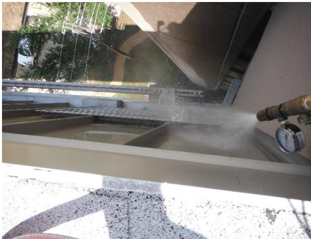
Figure 46. Water spray testing down onto the east facade louver near the Purple Garage. No water intrusion observed.
