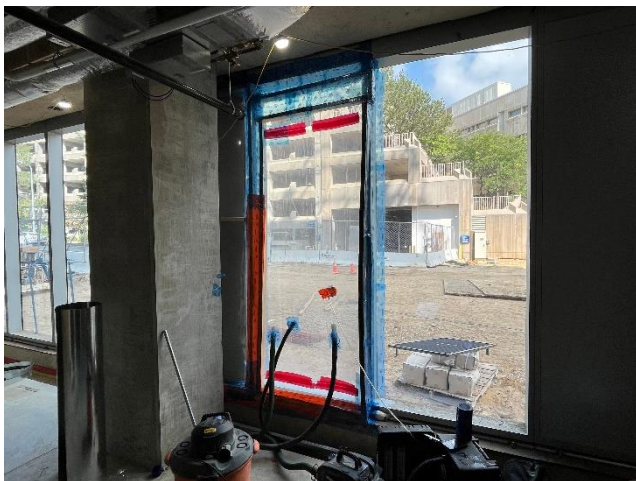
Photo 3 – Specimen 4, interior view of test chamber.
