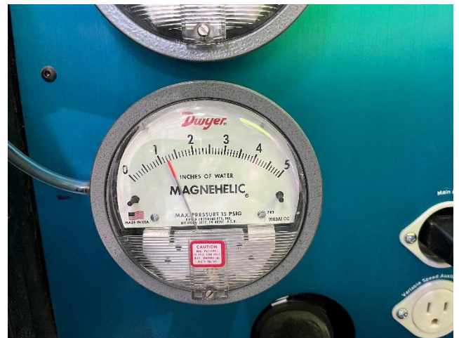
Photo 4 – Specimen 4 – Interior test chamber pressure at 1.2 in Aq.
