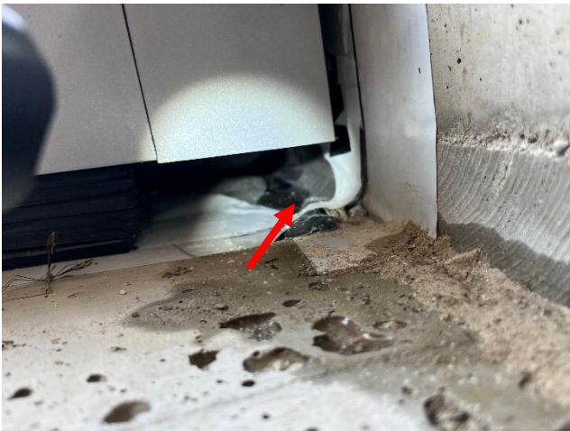
Photo 23 – View of Specimen 6 moisture intrusion at interior right sill/jamb interface.
