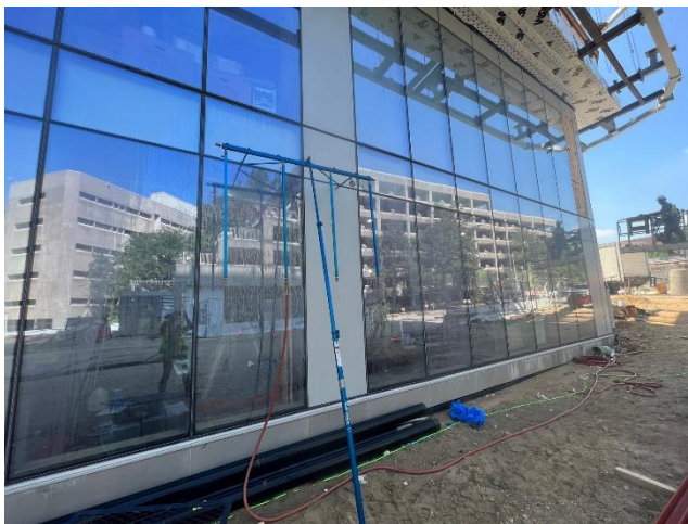
Photo 9 – Specimen 4, spray rack positioning at top of test area.
