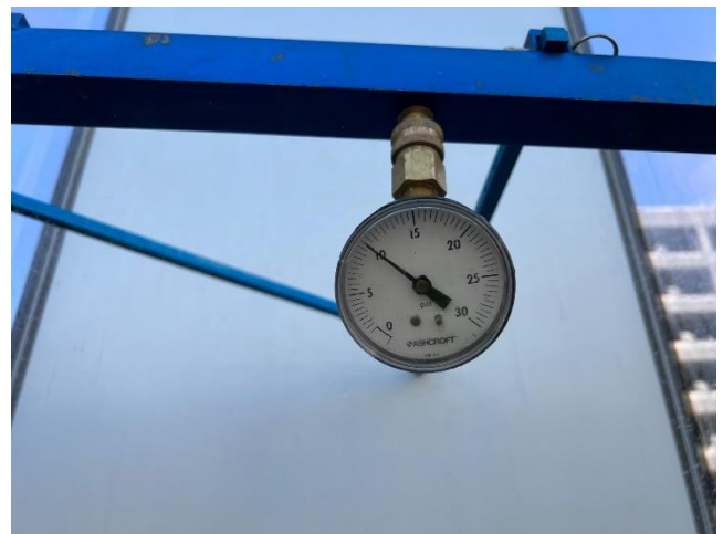
Photo 10 – Specimen 4, spray rack pressure at 10 psi.
