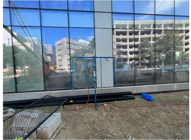
Photo 8 – Specimen 4, spray rack positioning at bottom of test area.
