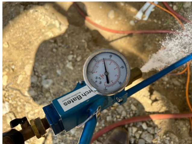
Photo 13 – Typical spray wand water pressure at 30 psi.
