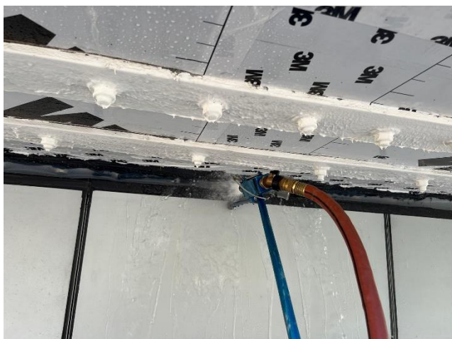
Photo 14 – Typical water spray application at Specimen 5.
