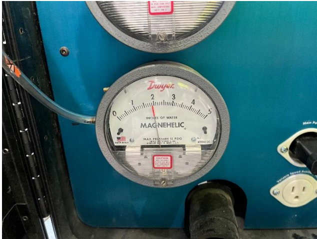
Photo 11 – Specimen 4, interior chamber pressure at 1.9 in Aq.
