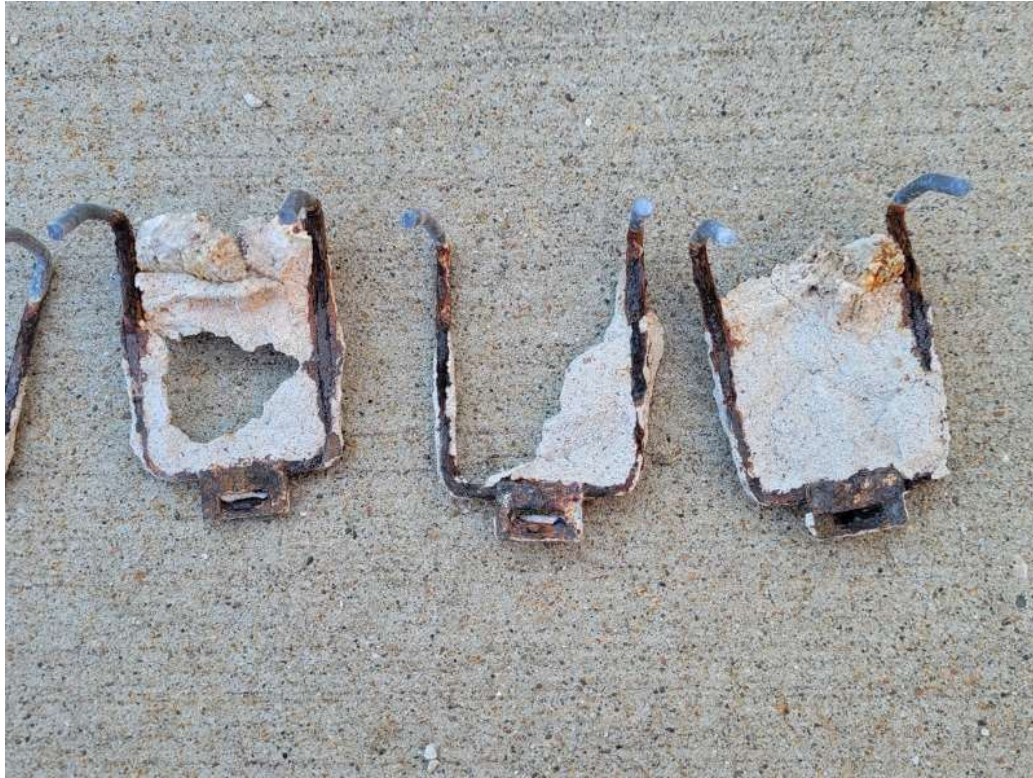
Photo #120: View of rusted brick anchor ties after removal from the wall (north elevation, fitness area, 6/27/23).
