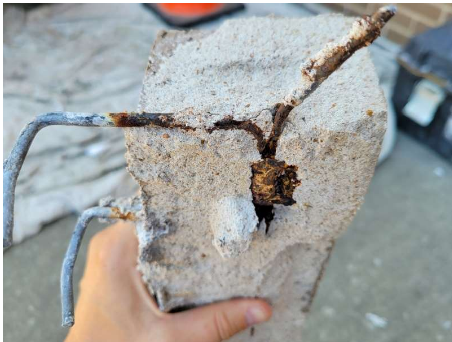
Photo #117: Underside view of a brick unit with a corroded brick anchor tie and wire, embedded in the mortar (north elevation, fitness area, 6/26/23).
